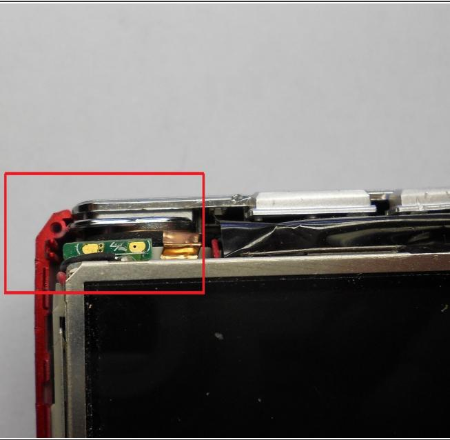
**⚠** This is where energy for the flash is stored. Even with batteries removed, if you touch these connections, you can be shocked, depending on if the flash capacitor has a stored charge. It may not have a stored charge, but work around this assuming it does.
