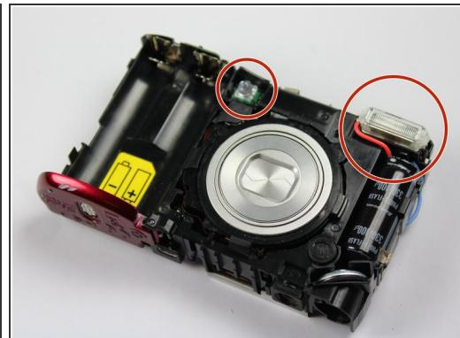
! Hold the camera with the lens face down to prevent the plastic covers of the warning light and the flash bulb from falling out.
