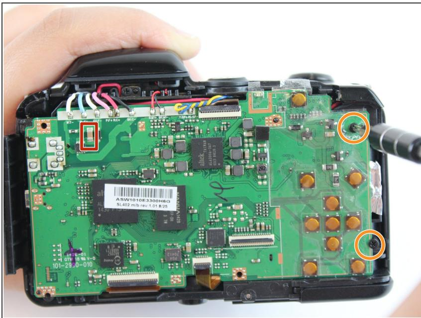
**⚠** The marked red box contains a highly charged capacitor. Check the charge using a voltmeter and discharge it first before continuing. [Discharge capacitor guide.](#)
