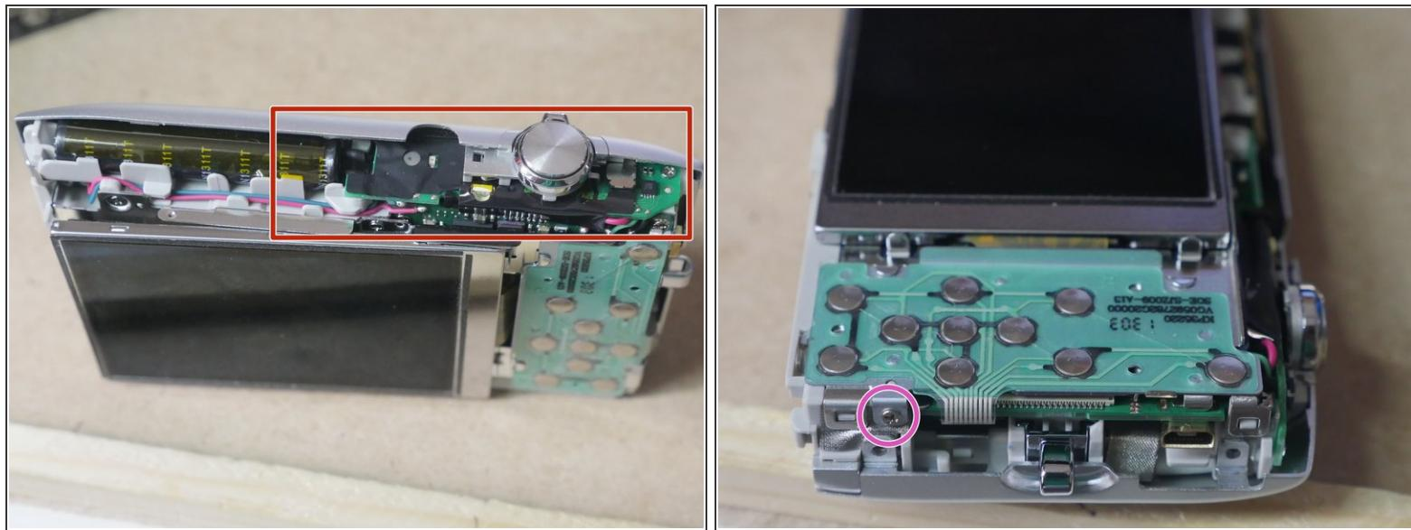
**⚠ Shock Hazard!** Do not touch anywhere along the top panel. Capacitor will still hold a residual charge that will shock you if touched. It is best to discharge the capacitor using the two metal solder joints on the top panel in front of the black tape
