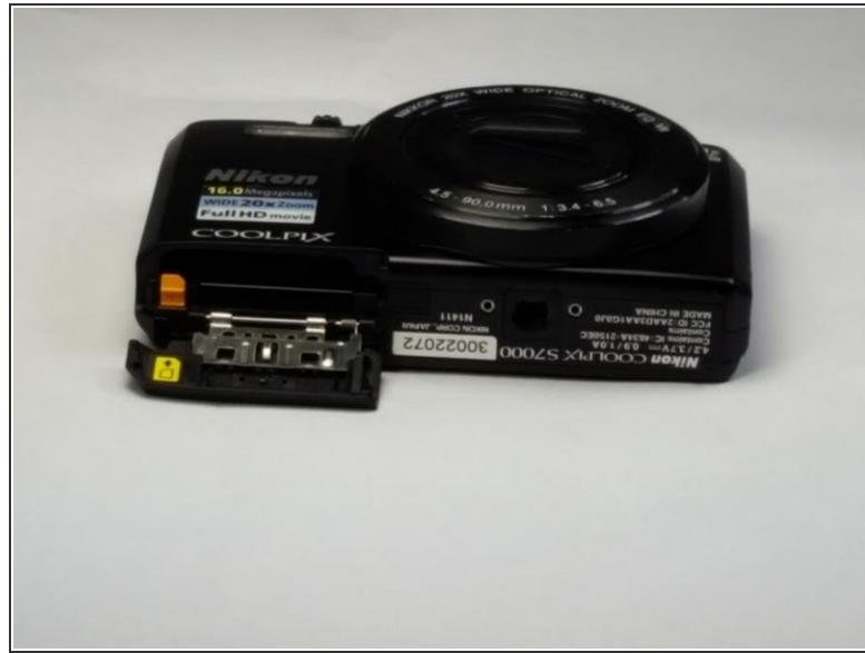
**⚠** Ensure that the camera is powered off to prevent damage during battery removal.
