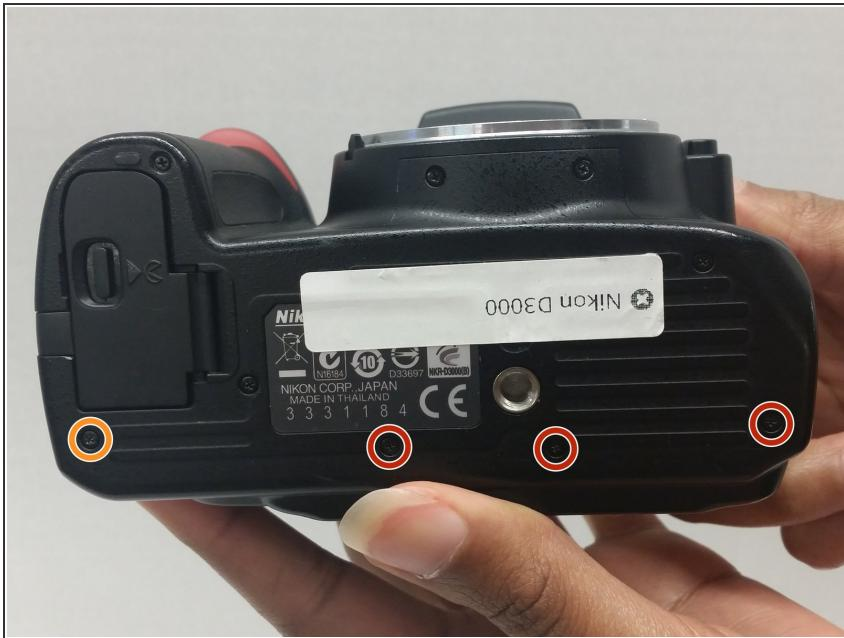
**i** Removal of the screws from the bottom will aid in the removal of the back as it loosens the bottom tabs of the camera back.
