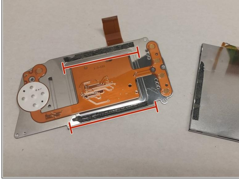
**⚠** Cover the old LCD Screen with tape before removing to avoid broken glass if the screen cracks during removal.
