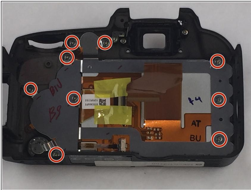
⚠ Be careful when separating the metal plate from the back panel because the speaker wire is connected to the metal plate. It can easily be torn if caution is not taken.
