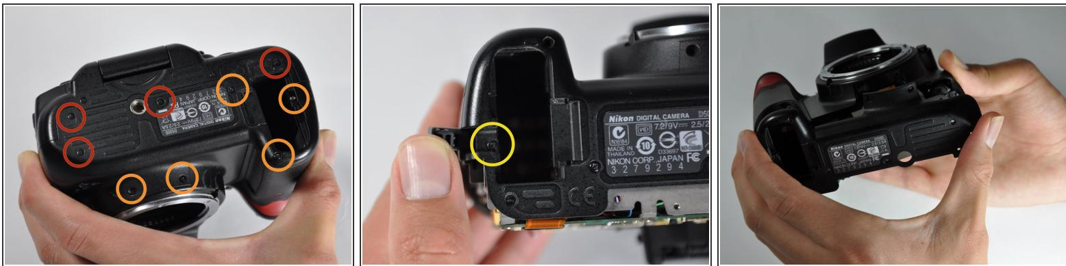
*(i)* The viewfinder is held on by the top body piece. To access it, the entire plastic body must be removed. Each piece (back, bottom, front, top) helps secure the next piece.
