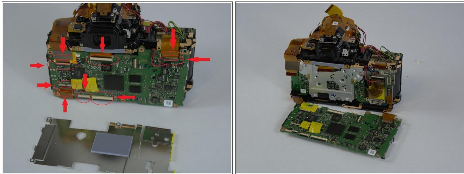
*(i)* The six screws that were removed in the previous step also hold the motherboard in place.
