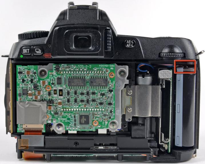
⚠ At this point, the capacitor is visible and its exposed contacts are boxed in red. Even though they are recessed, be careful not to touch the contacts to avoid shocking yourself.
