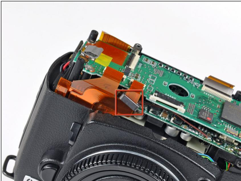
↗ Be sure not to lose the small iron core around the DC-In ribbon cable.
