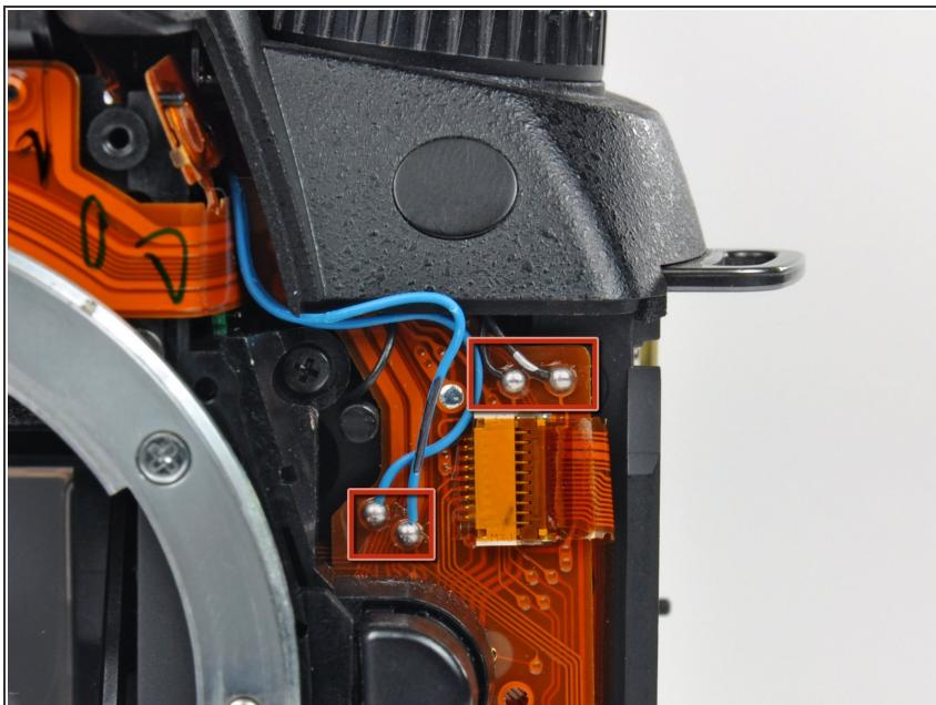
**i** In this step, you will de-solder the four wires pictured. Mark the wires with a sharpie or a paint marker to keep track of their locations, as each pair of leads is nearly identical.
