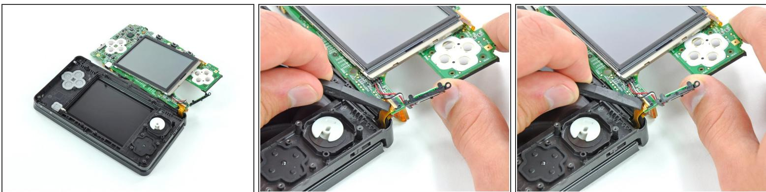
ⓘ Continue lifting the motherboard assembly and rotate it until it is resting next to the rest of the device.
