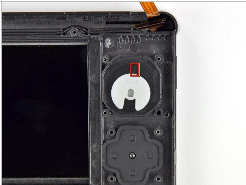
*i* There is a black plastic ring that sits between the bottom of the circle pad and the underside of the upper case.
