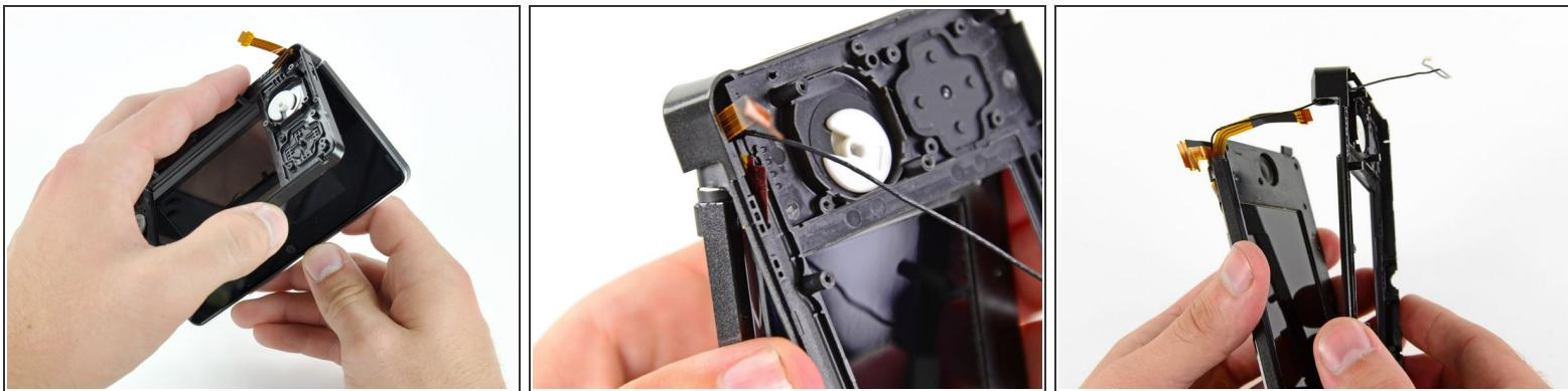
**⚠** Before proceeding, note how the 3 ribbon cables are oriented (what direction the gold contacts face) and layered together (which cable is on top of which). The cables are too short to reach if they are threaded through in any other orientation.
