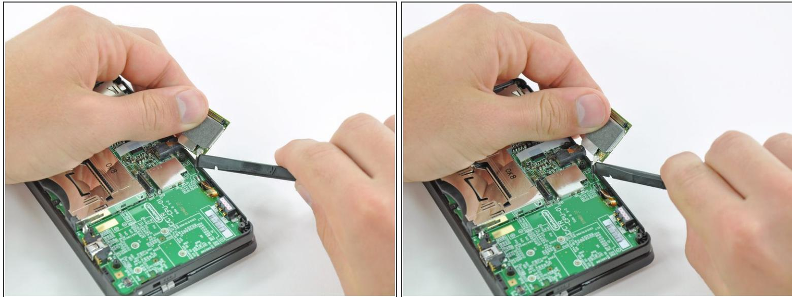
*(i)* Lift the Wi-Fi board off the motherboard and rotate it so that the bottom side is facing up.
