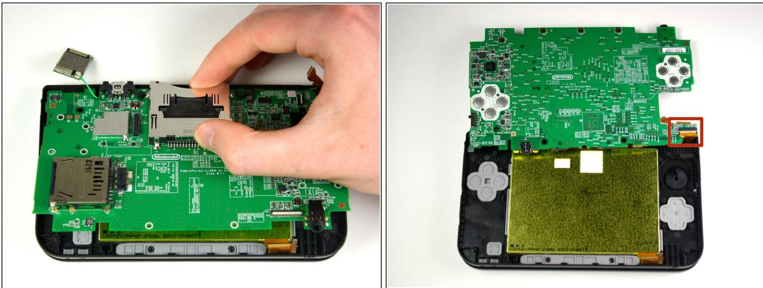
! The motherboard will still be attached at the top right hand corner so do not completely detach it at this point.
