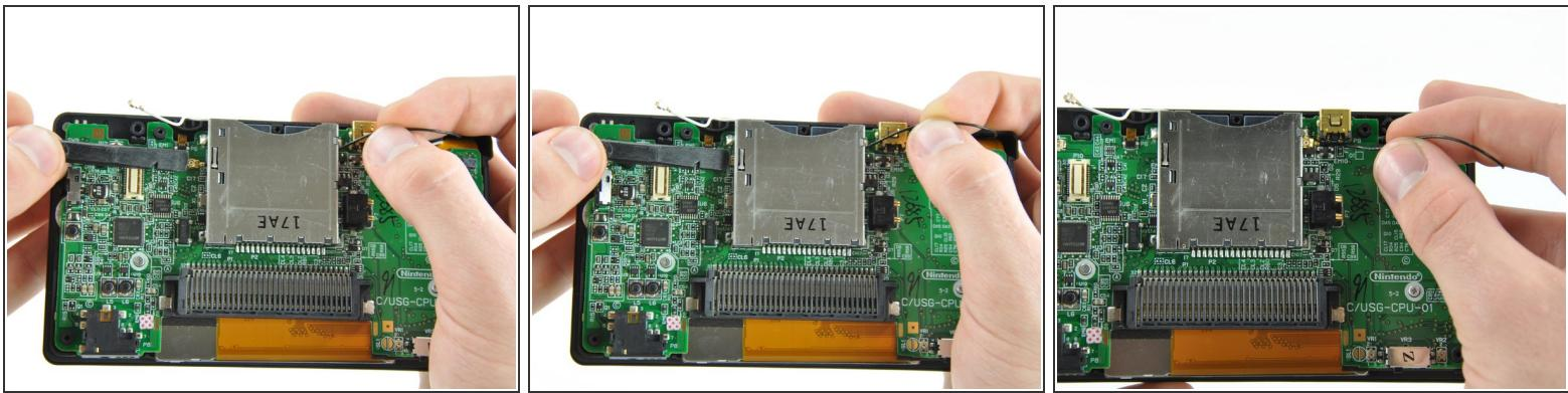
**⚠** In the following steps you must pull the antenna cable between the DS Lite game cartridge reader and motherboard. Pull slowly and stop when you feel resistance to avoid damaging the cable or motherboard.
