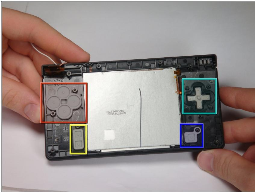
★ Remove the rubber front-panel button membranes from the device. Pay careful attention to where the buttons go, so you can replace them correctly.
