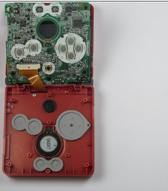
**⚠** Be careful not to tear the ribbon cable that's connected to the screen. If you tear it, games will not appear on the device's screen!
