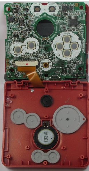
**⚠** Be careful not to tear the ribbon cable that's connected to the screen. If you tear it, games will not appear on the device's screen!
