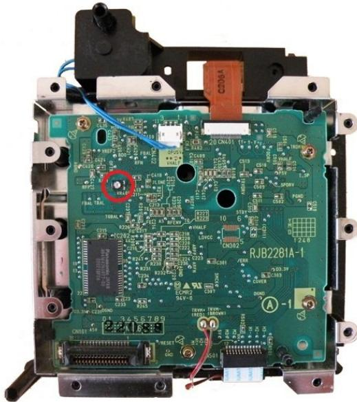
**i** The potentiometer is located as shown in the picture. It's a very small cross-wing screw mounted on top of a little black box.
