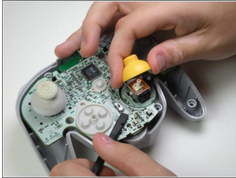
⚠ Rough handling of the C-stick could cause the daughter board to break off of the motherboard.
