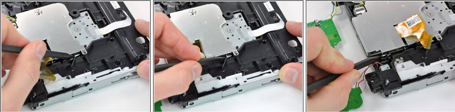
ⓘ The side of the EMI shield with the slot for the DVD lens ribbon cable has two small metal clips that fasten to black plastic tabs on the DVD drive housing.
