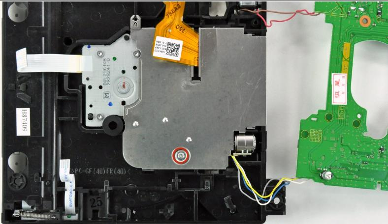
ⓘ Lay the DVD drive board next to the DVD drive in such a manner that the cables soldered to the DVD drive board are out of the way (as shown in the picture)
