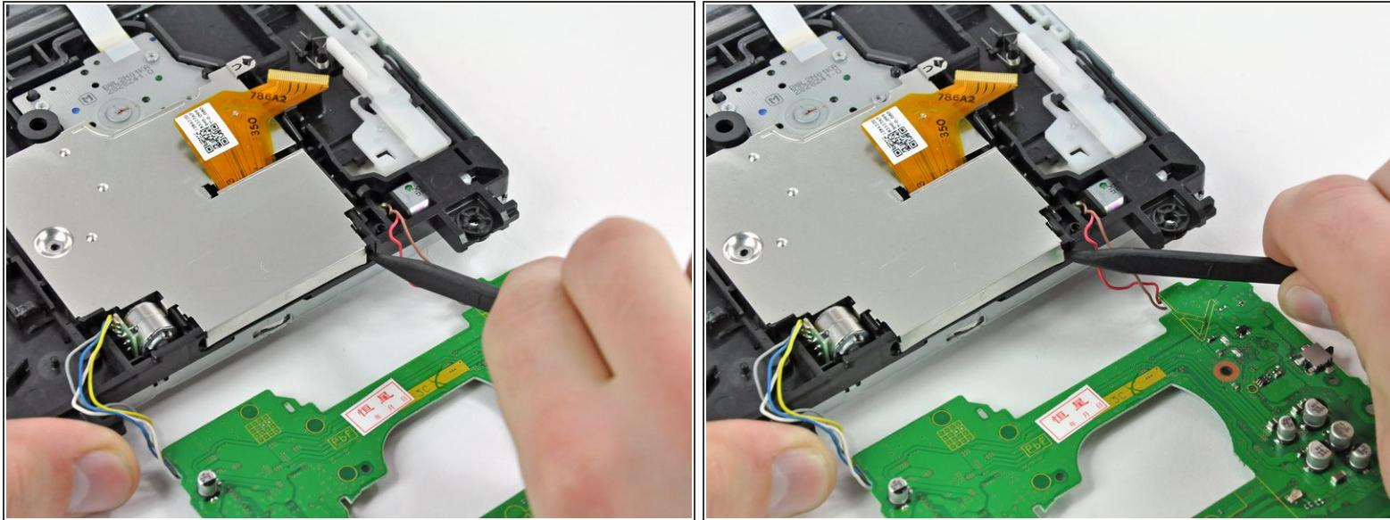
*(i)* Small tabs on the EMI shield sit in two holes on the outside edge of the DVD drive housing.
