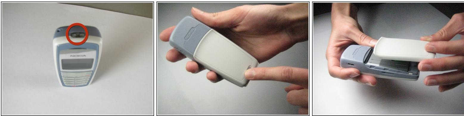
**⚠** To prevent shock, press down on the power button located on the top of the phone until the phone shuts off.
