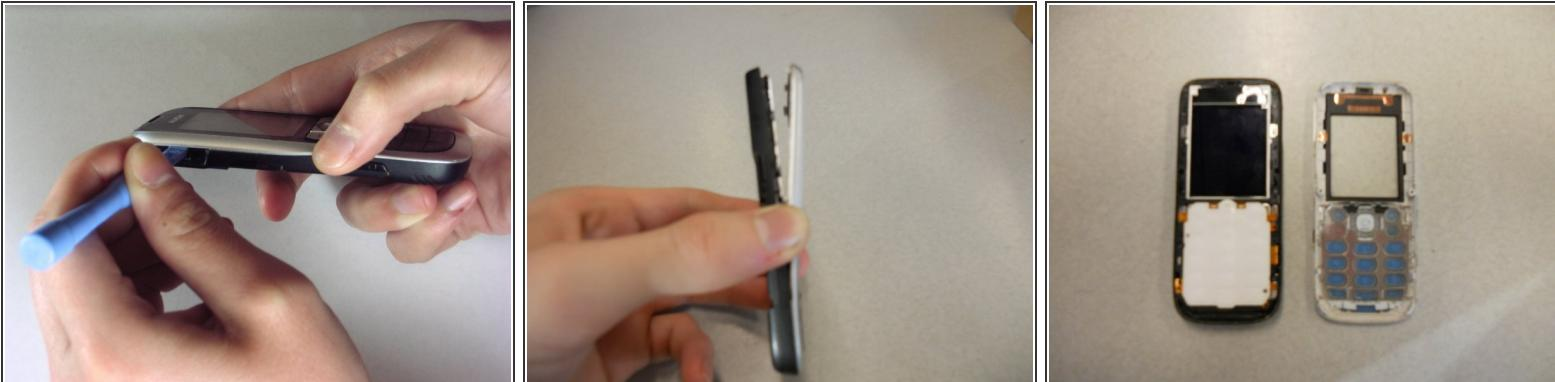
**⚠** Separate the front case from the back case using the iPod opener
