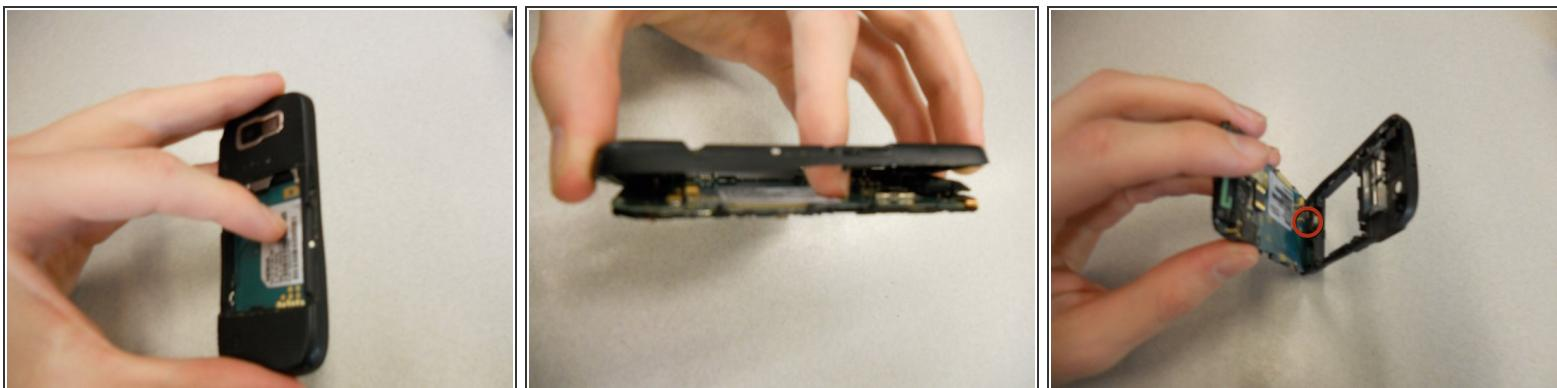
! DO NOT PULL APART! There is a wire attaching the speaker to the rear case. It is very important to NOT sever this connection. Because of this, the rear case does not completely detach from the rest of the phone.
