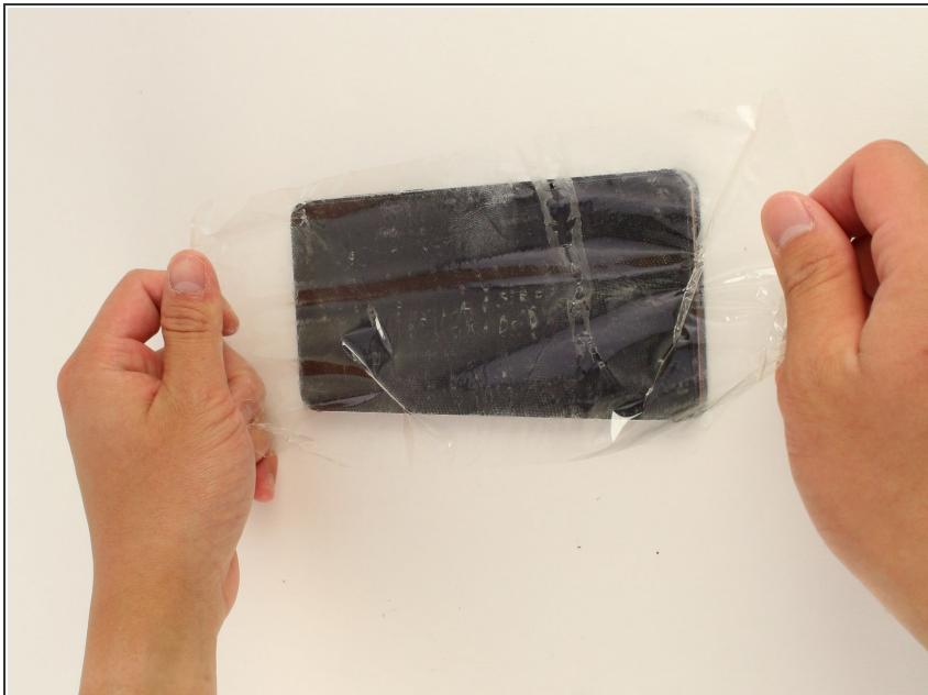
⚠ If your display glass is cracked, take precaution by taping over the display to prevent further breakage and harm.
