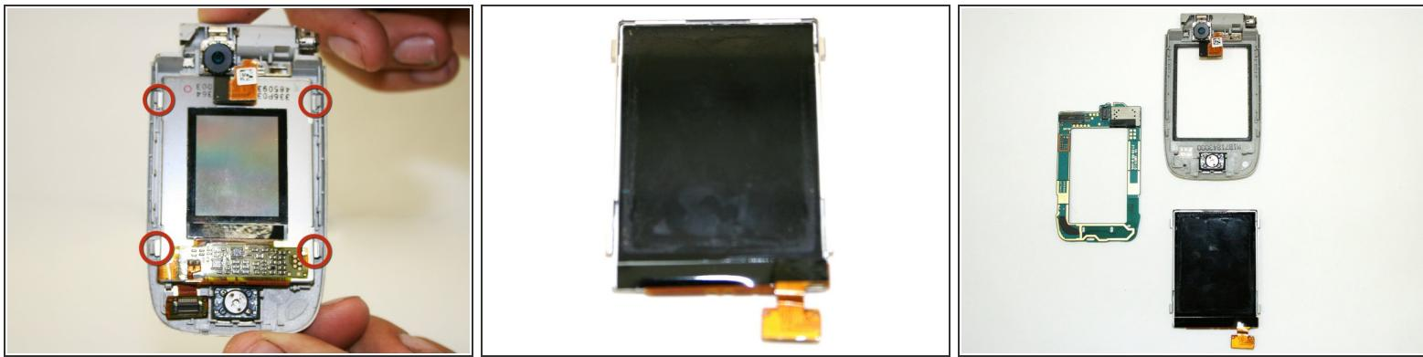
**⚠** Pry back the associated tabs using your thumbnail or an iPod opening tool by pulling them away from the LCD panel.
