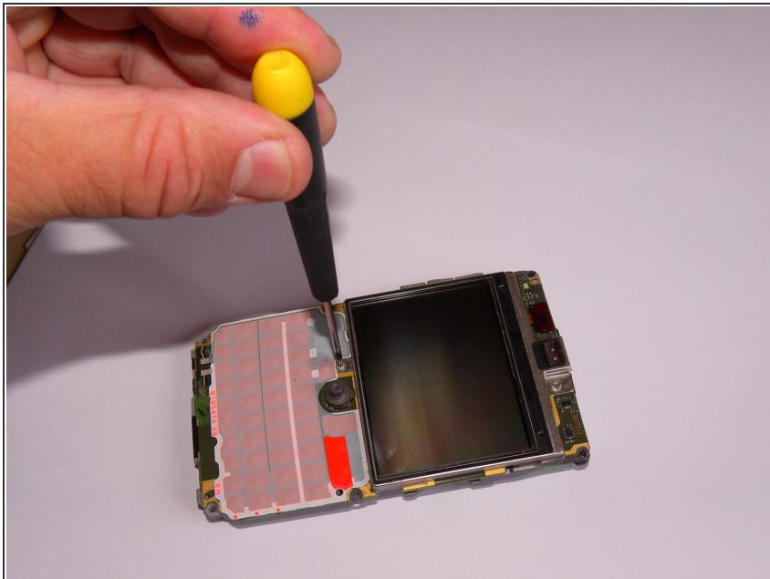
**⚠ CAUTION!** Remove the bottom screw with T5 Torx screw driver, not T6 !
