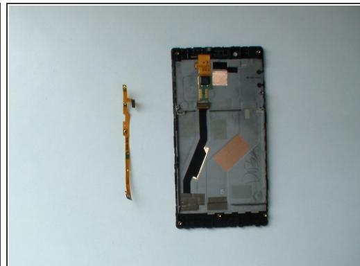
! When you start with the removing the ribbon cable be careful with the buttons and with the small black cups on it.
