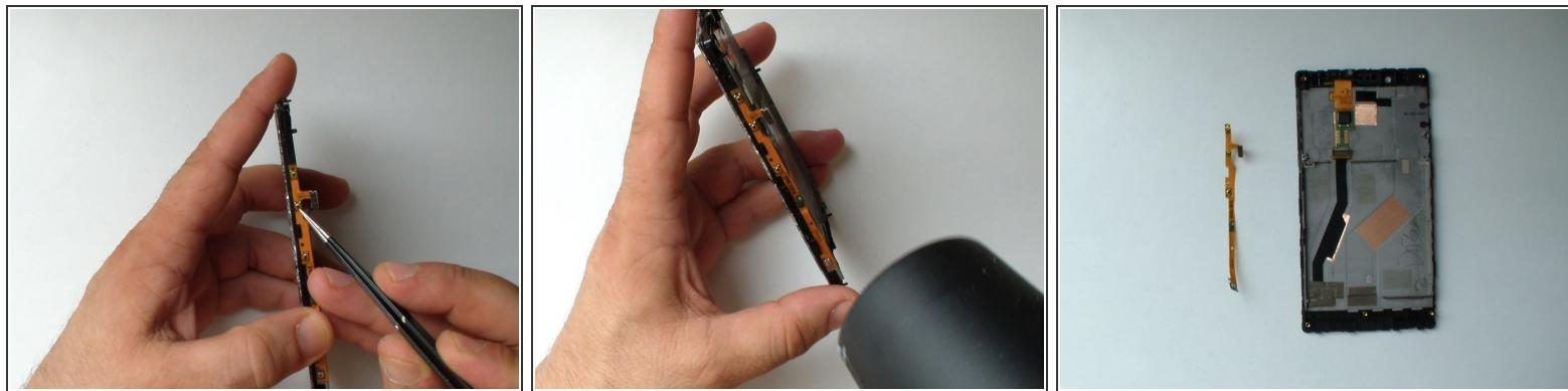
**⚠** When you start with the removing the ribbon cable be careful with the buttons and with the small black cups on it.
