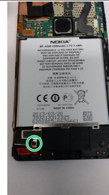
ⓘ We're going to remove all screws in one step now. Please make sure to place them in a way that you know how to screw them back in place when reassembling the device. If you interchange the screws this might cause damage to your device.
