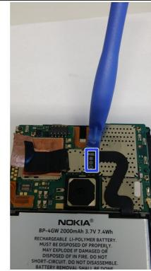
**⚠** Don't remove the back cover completely yet because it's still attached with a ribbon cable which you can easily rip apart.
