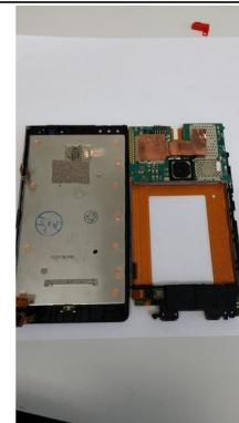
**⚠** During this step, some components may fall out of their place, such as the speaker or SIM card cover, but you can easily put them back by slightly lifting up the logic board.
