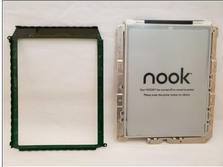
⚠ The display cracks very easily. If this happens, there will be glass shards that could potentially cause injury. You may want to wear protection for hands and eyes while completing this step.
