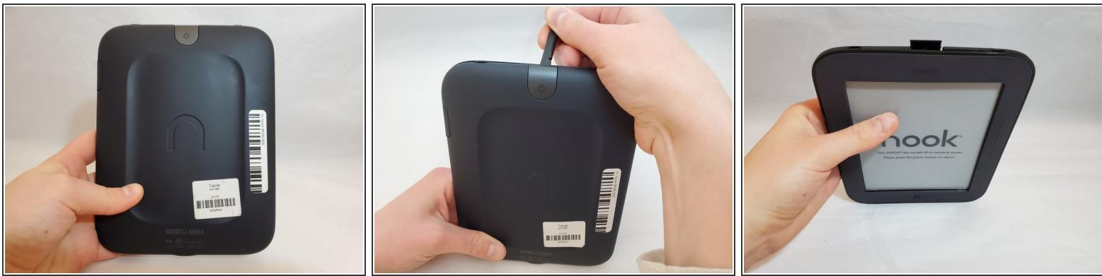
! Power off your Nook before working on your device. Hold the power button for about 5 seconds and select the “Power Off” option.
