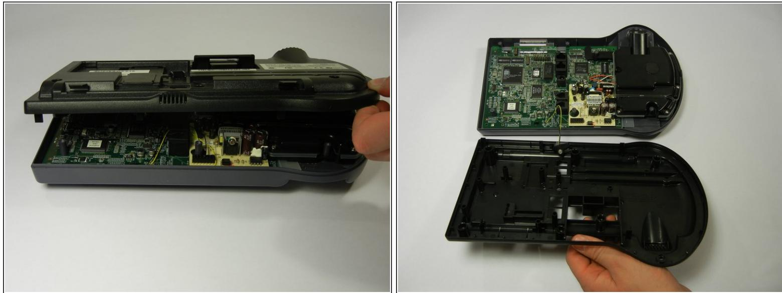
**⚠** Lift up the back cover slowly because there are still wires attached to the circuit board.
