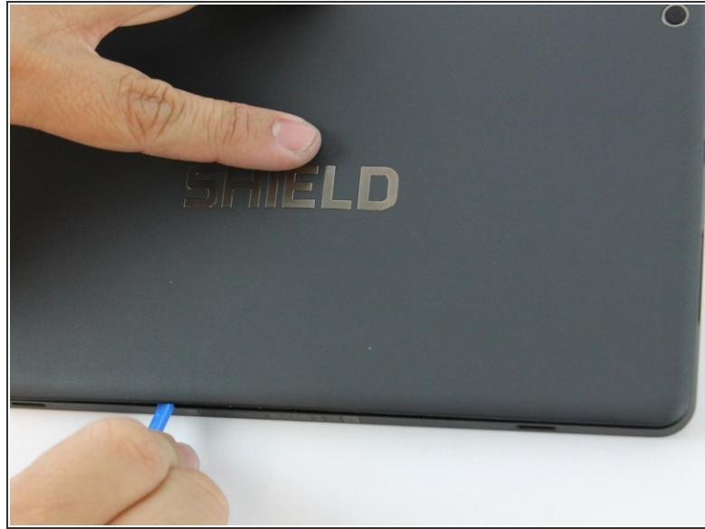
★ There are clips holding the back panel to the rest of the case. You must apply some force to lift the back panel off.
