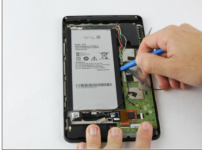
! The battery is heavily glued down so you will need to apply force while also exercising caution to not damage the rest of the device.
