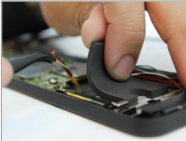
**⚠** The audio input film is running underneath the foam piece and is fragile. Be careful when removing this piece.
