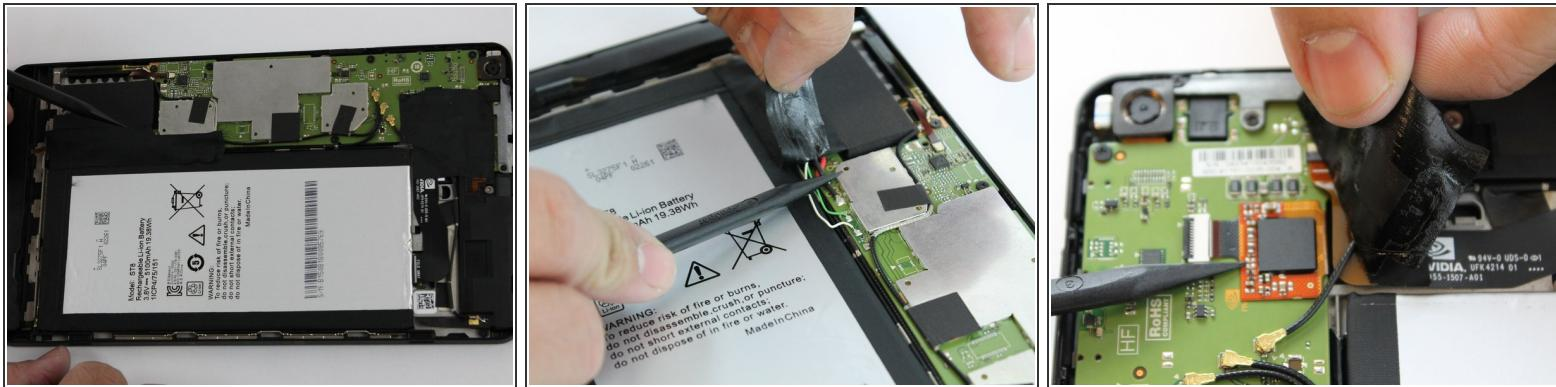
**⚠** Be careful when removing the two pieces of tape because there are wires underneath the tape.
