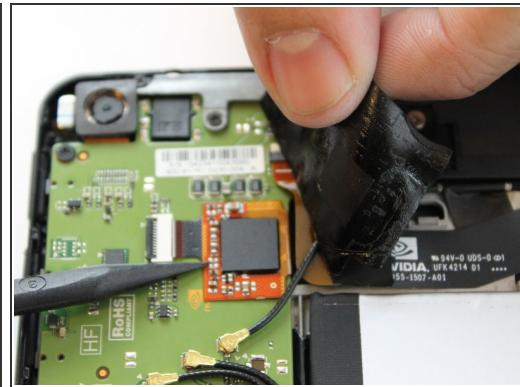
**⚠** Be careful when removing the two pieces of tape because there are wires underneath the tape. Lifting too hard may accidentally rip out the wires.
