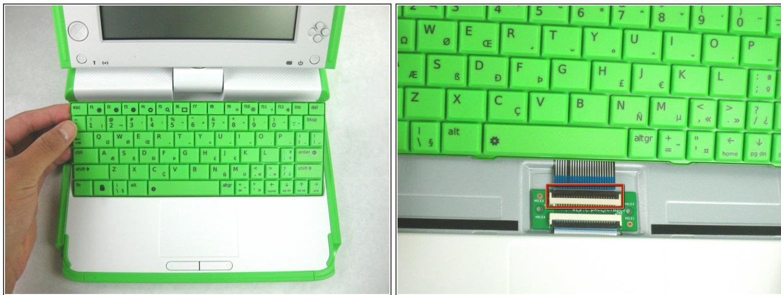
! Be careful not to pull the keyboard too far because there is still a ribbon cable attached to the bottom.
