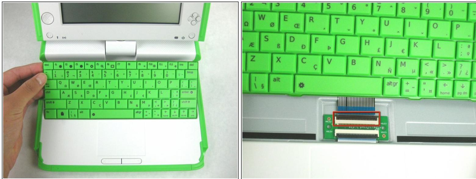
! Be careful not to pull the keyboard too far because there is still a ribbon cable attached to the bottom.
