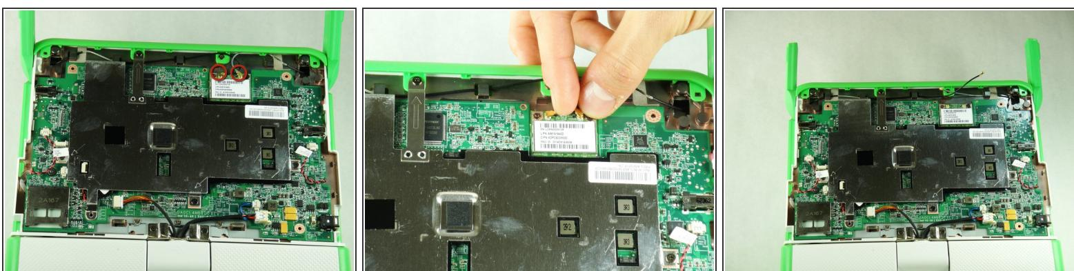
⚠ When pulling out the connectors, make sure to hold the metal connector instead of the wire.
