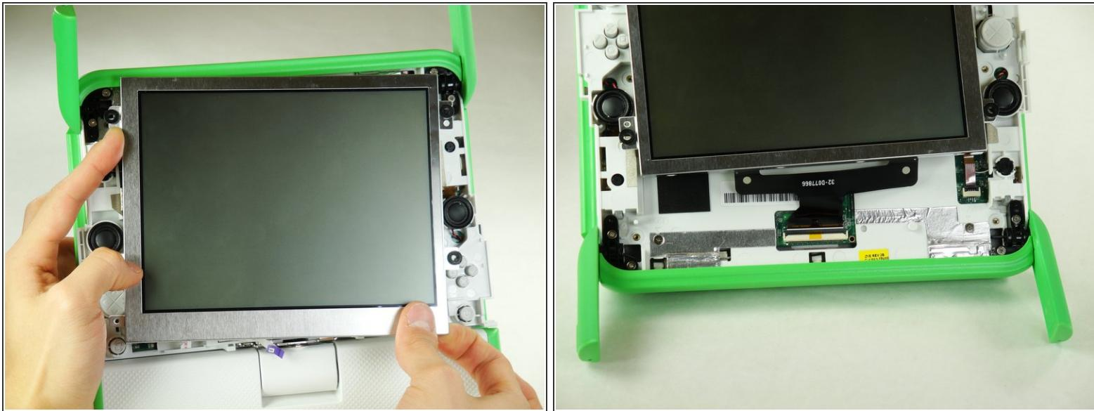
**⚠** Be careful not to pull the screen out too far. There are two ribbon cables attached to the screen, and they can easily break.
