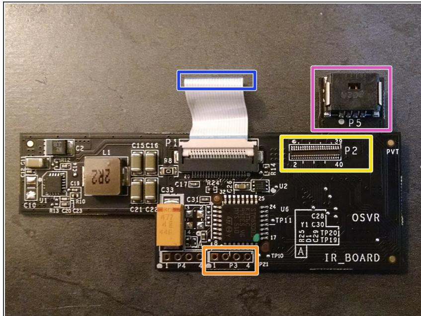
**i** This is a view of a HDK v1.4 and up IR board, looking at the side that faces the outside of the HMD. When re-installed, the left edge of the board as seen here goes toward the top of the HMD.
