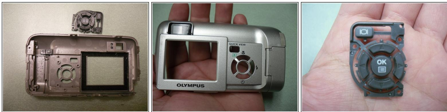
*(i)* The button assembly is now separate from the back cover.
