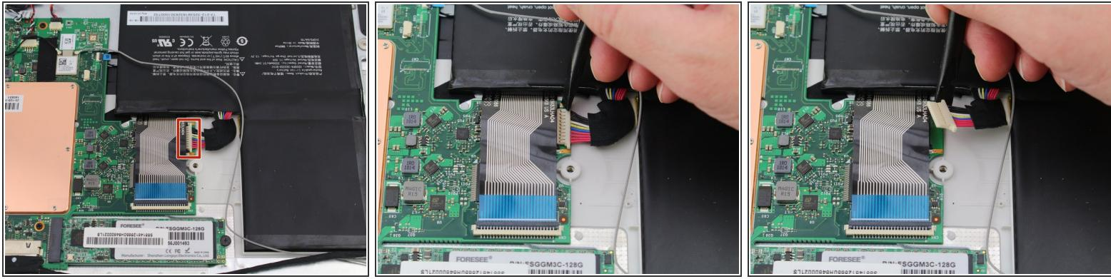
*(i)* There may be black tape inside your device covering components or holding down wires. This tape is unimportant for the function of the device, and can be removed.
