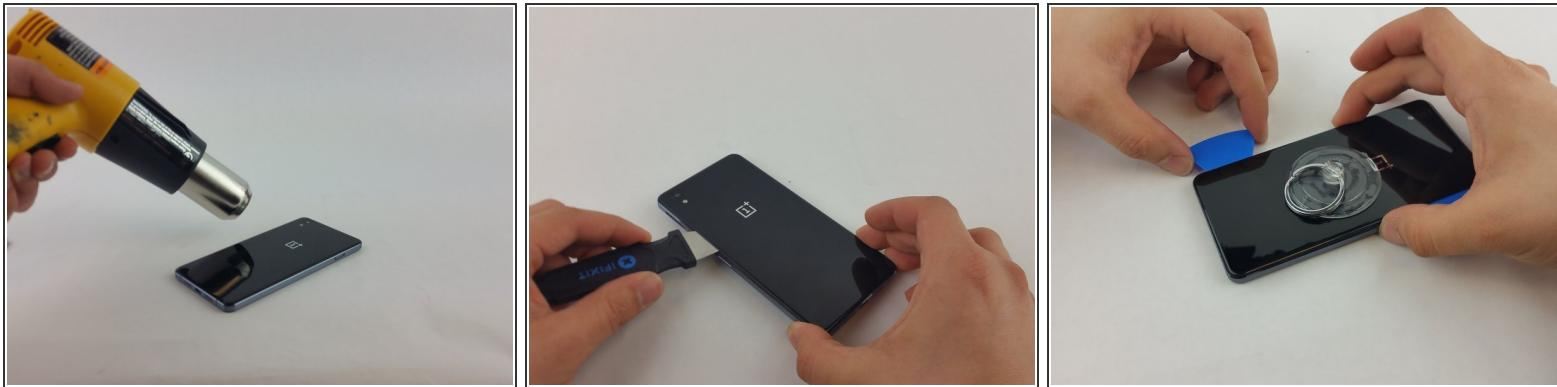
**⚠** Put on heat-resistant gloves and place the phone on a surface that will not catch fire or melt.
