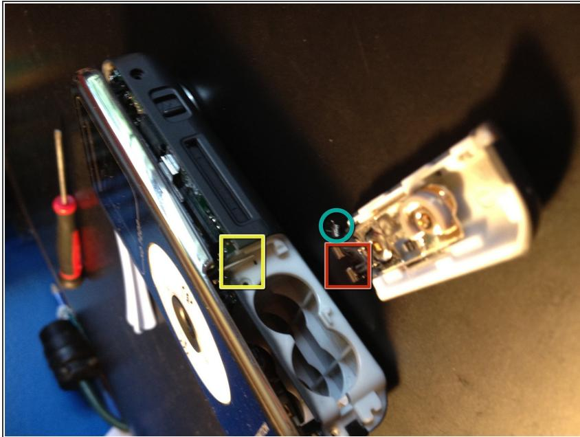
⚠ When lifting the front off the hatch for the batteries will come off. when putting it back together put the spring (in green) in between the rail holders (in red) then slip it on the rail (yellow).
