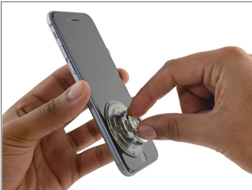
**i** Opening the display on the 6s separates a thin strip of adhesive around the perimeter of the display. If you prefer to replace the adhesive, have a set of new adhesive strips ready before you continue. It's possible to complete the repair without replacing the adhesive, and you probably won't notice any difference in functionality.
