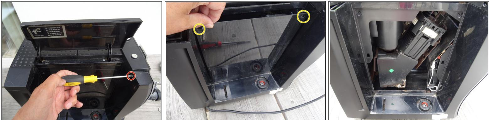
*(i)* In this step, you should remove the screws of the right side panel. The side panel itself can only be removed after removing the top cover.
