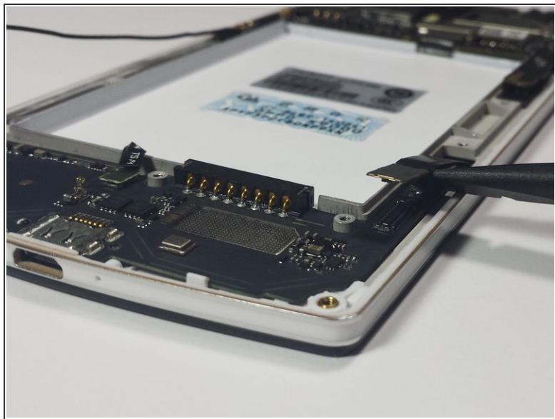
**⚠** Like the last step, this connection is tricky to remove. Please pay close attention to the guide to avoid damaging your device.
